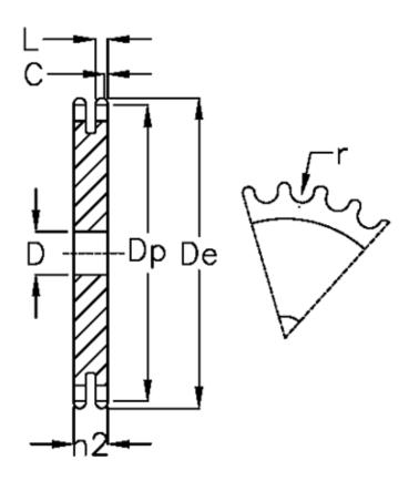
C = 4 D = 25 De = 298.7 Dp = 283.56 For chain size = 1 1/4 x 3/4 For chain type = 20 B-2 h2 = 54.6 L = 18.2
